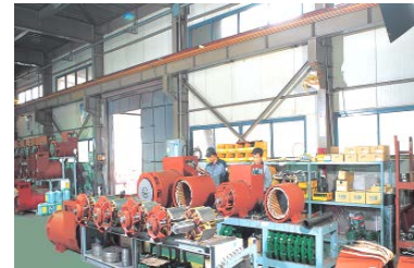
ALTERNATOR ASSEMBLING
